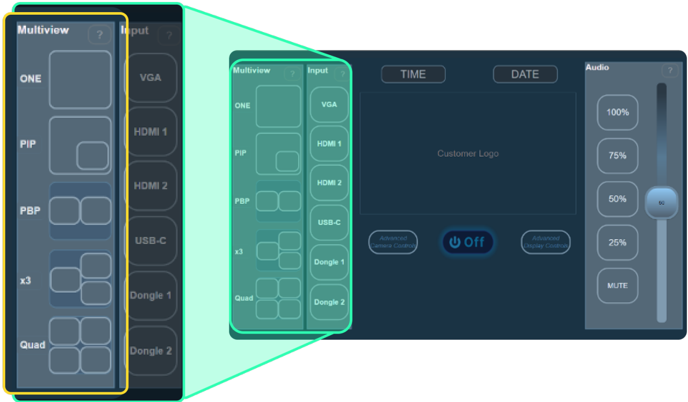
Source zones are the areas where the input will be displayed on the screen
